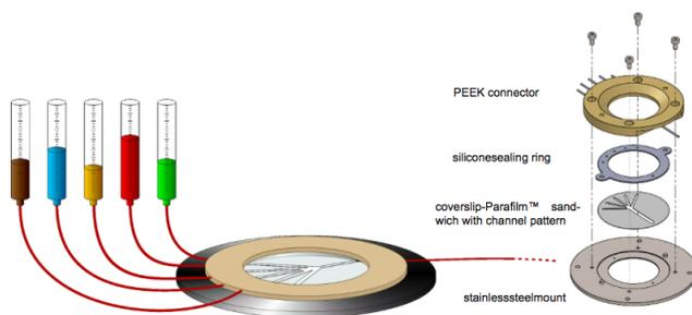
**Figure 2.** The schematic illustrates the assembly of the LaminarFlowCell and the geometry in which up to five laminar flows are generated from various syringes.
