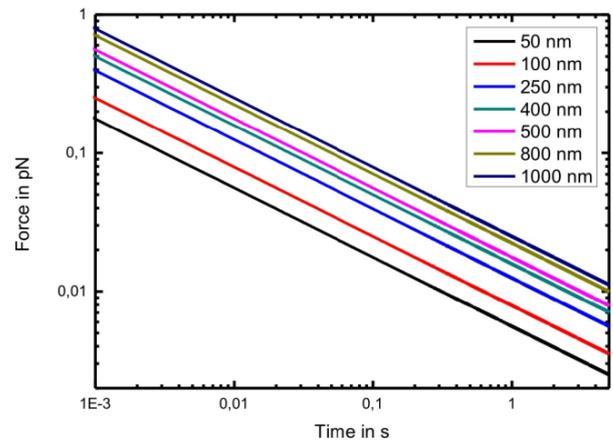
**Figure 6** Smallest force that can be measured in a time  $t$  with particles of different diameters.
