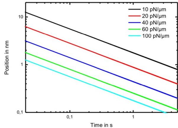
**Figure 5** Smallest displacement that can be measured for a trapped particle with a diameter of 1000 nm at various trap stiffnesses.
