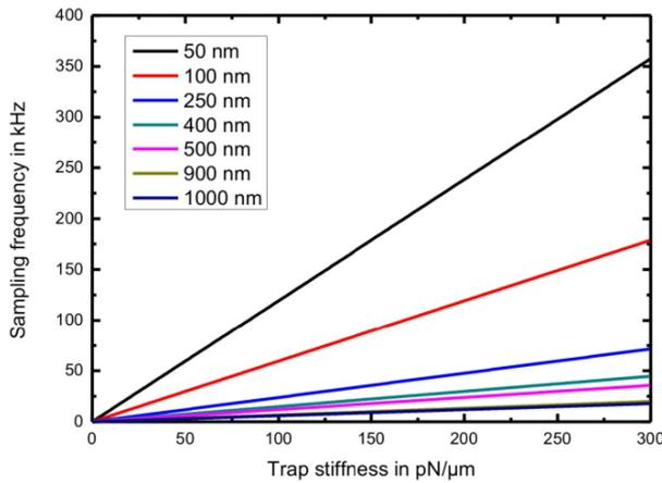
**Figure 8** Highest useful sampling frequency if only events slower than the auto-correlation time are to be measured (for different particle diameters).
