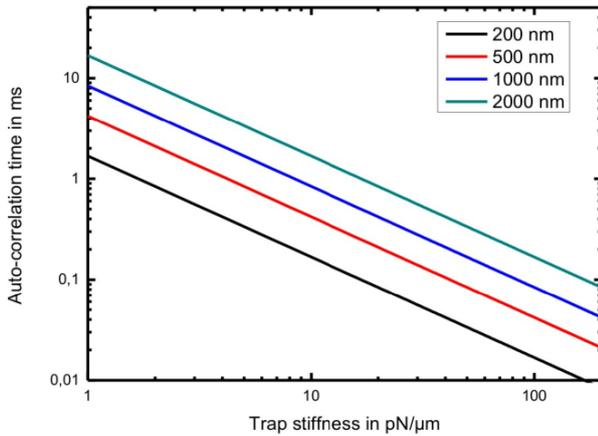
**Figure 2** Auto-correlation time for trap stiffness values ranging from 1 pN/μm to 200 pN/μm calculated for four different bead diameters.
