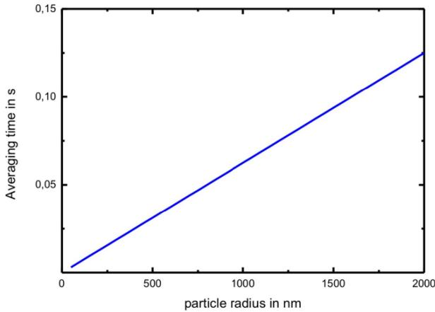
**Figure 7** Time necessary to significantly measure a force of 100 fN acting on a particle.
