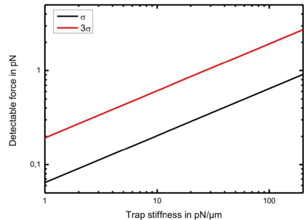
**Figure 4** Achievable force resolution (up to 68.3% and 99.7% accuracy, respectively) as a function of trap stiffness for a single measurement.
