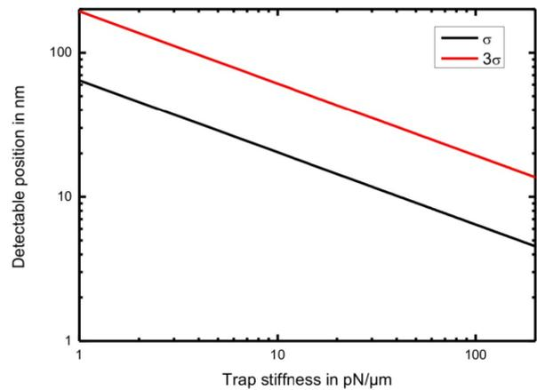
**Figure 3** Spatial accuracy (up to 68.3% and 99.7% accuracy, respectively) for measurements with a particle undergoing Brownian movement within an optical trap as a function of trap stiffness.
