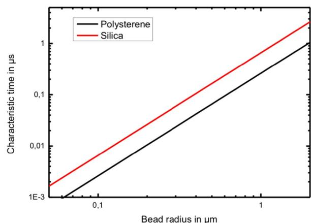
**Figure 1** Characteristic time for polystyrene and silica particles with diameters between 10 nm and 4  $\mu\text{m}$  as typically used in experiments with optical tweezers.
