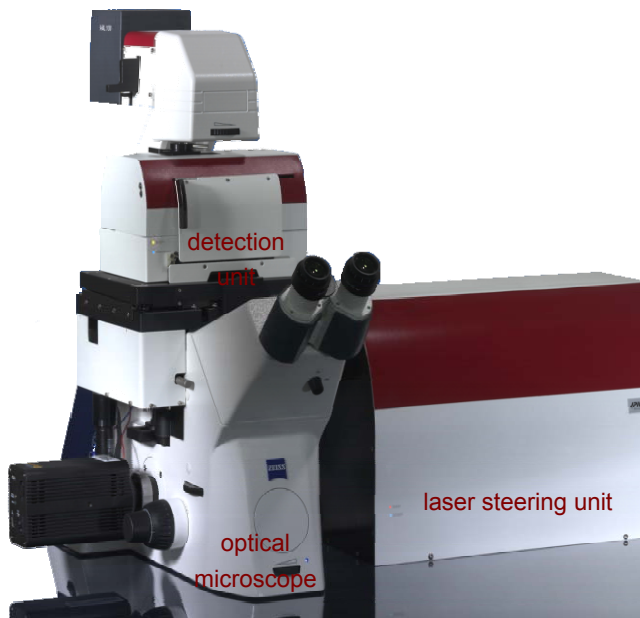
Fig. 2: The JPK NanoTracker™ optical tweezers platform, including the laser steering unit, the optical microscope and the detection unit.
