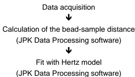
The Hertz model is applied to describe the indentation of an elastic half-space and a sphere. These assumptions can be made for sample surfaces and volumes much bigger than the bead used for the indentation. It relates force  $F$  and indentation depth  $\delta$  as follows:
