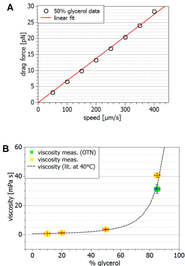
**Figure 1 Viscous drag measurements in glycerol water mixture.** **A** The viscous drag force  $F_d$  is measured at different flow speeds  $v$ . The red line represents a fit of the linear relation of the Stokes equation (1). With this, the viscosity  $\eta$  can be derived. **B** Measurements of  $\eta$  for water mixtures with increasing glycerol content. The yellow squares represent measurements based on a trap calibration in water.
