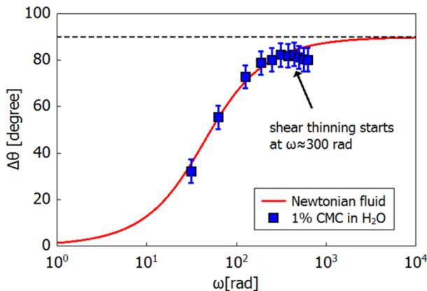
**Figure 5 Frequency dependence of the phase shift in 1% carboxy-methylcellulose (CMC) solution.** The phase difference  $\Delta\theta$  increases with increasing (angular) frequencies. At approx. 300 rad, the behavior deviates from that of a purely viscous Newtonian fluid, due to the shear thinning effect. The filaments in the polymer solution disentangle at these rates, which influences the mechanical properties of the material.
