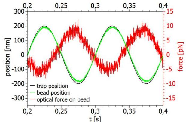
**Figure 4 Active micro-rheology.** A trap holding a PS bead performs a sinusoidal movement with  $f = 10 \text{ Hz}$  and  $200 \text{ nm}$  amplitude. The oscillations of the trap (black) and bead (green) position, as well as the force (red), are phase shifted. The magnitude of the shift changes with increasing frequencies and is characteristic for the viscoelastic properties of the fluid.
