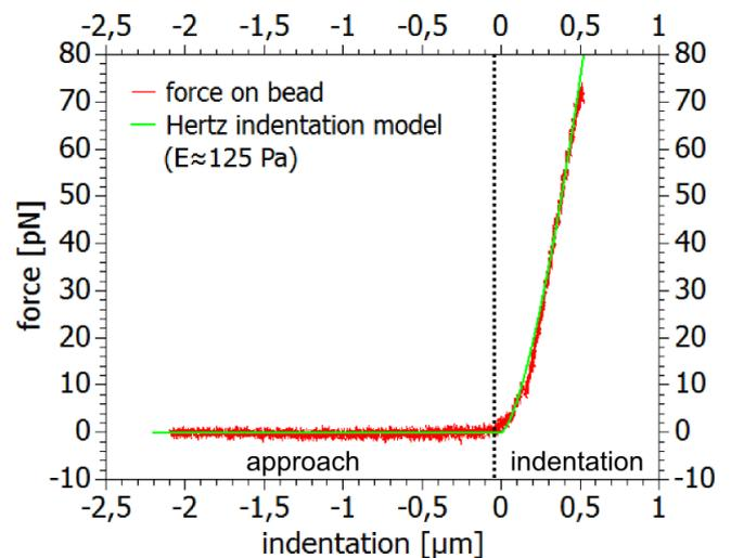
**Figure 3 Elasticity measurements using the Hertz model.** The measured force-indentation data (red curve) was fitted with the Hertz model (green) taking into account the shape and size of the indenting particle. The calculated Young's modulus  $E$  for the sample is 125 Pa.
