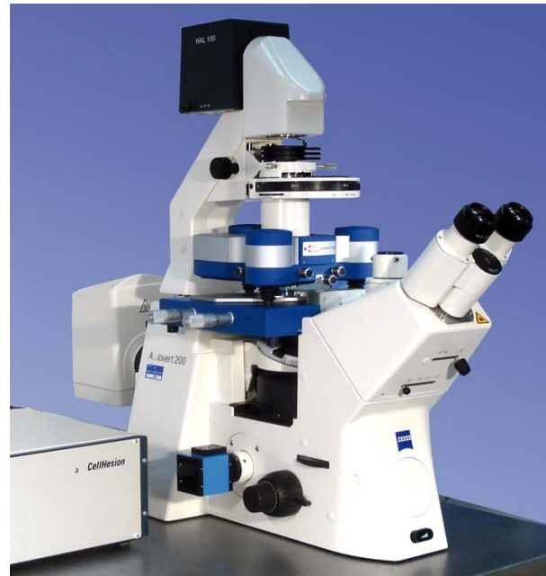
Fig. 2 The CellHesion® module. The CellHesion® module is an add-on to the NanoWizard AFM. The setup is integrated into an inverted light microscope for easy handling and to extend the scope of possible experiments.
