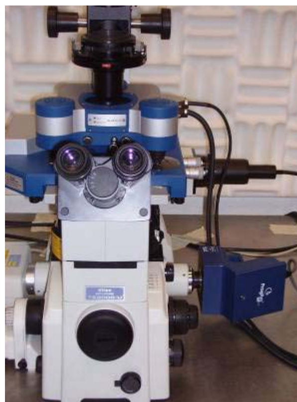
Fig. 1: Fluorescence setup (Nikon Eclipse TE2000) with the ProgRes® MF cool camera and the JPK NanoWizard®II.
